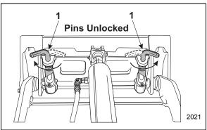
Figure 3-25 Attachment Locks in Unlocked Position
